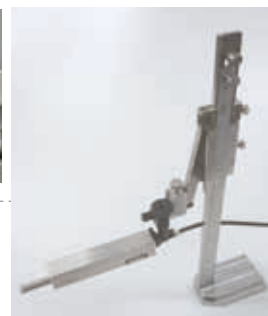
Sample combination of a tracing driver and height gage
