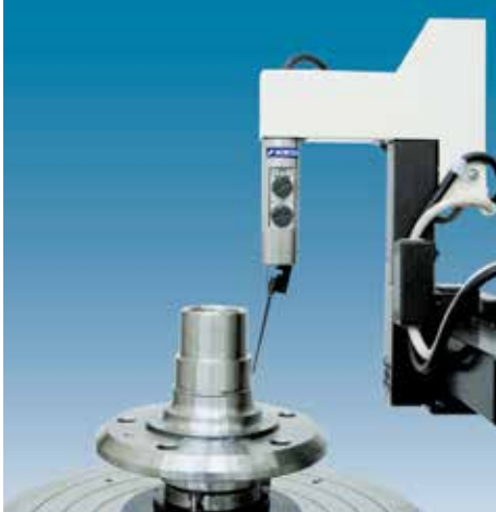
Sample roundness measurement of outside diameter
