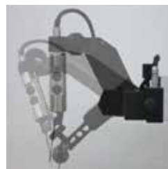
Example of effective workpiece measurement with the offset type detector holder
