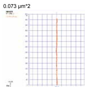
Vertical direction straightness (Using a straight edge) *2 Value after separation of straightedge accuracy
