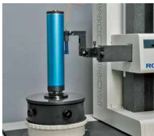
Sample of roundness measurement using a non-contact detector (option)
