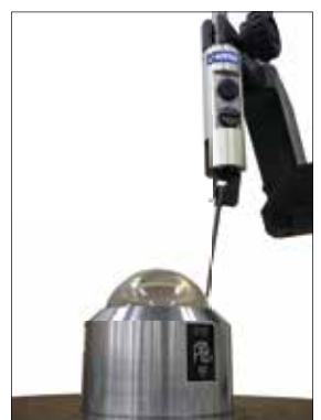
Roundness (Using a master ball) *1 Value after separation of master ball accuracy
